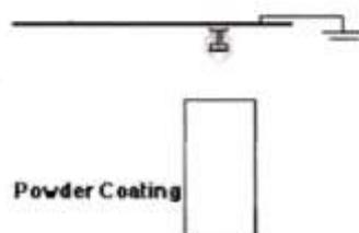
The powder is applied with an electrostatic spray gun to a part that is at earth (or ground) potential.
