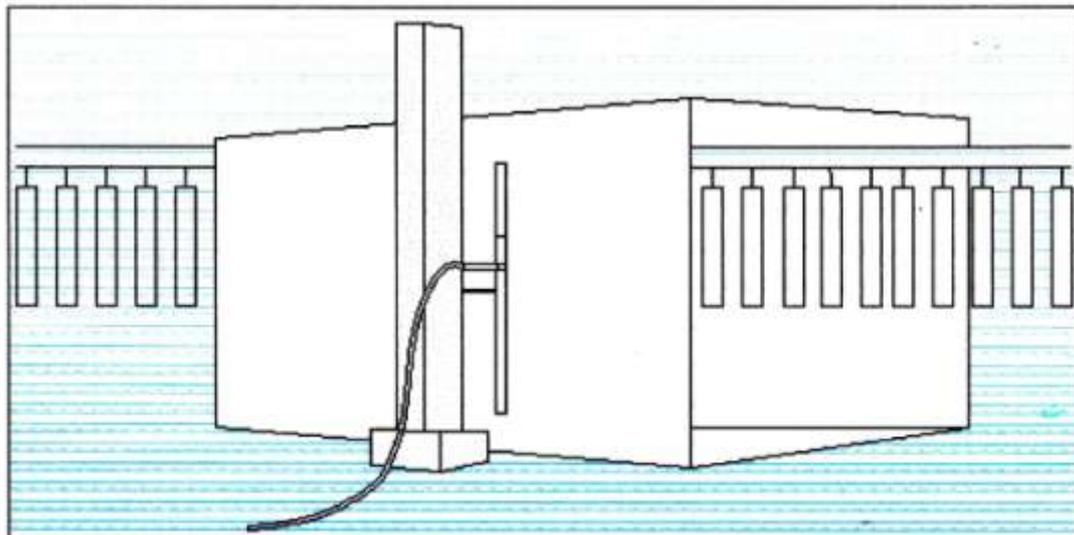
Normally some of the powder guns are in fixed position, while the most of the guns move automatically slowly up and down. Adjustment of the guns is – as mentioned above – dependent on the shape of the profile, but also dependent on which coating thickness and finish which are requested.
