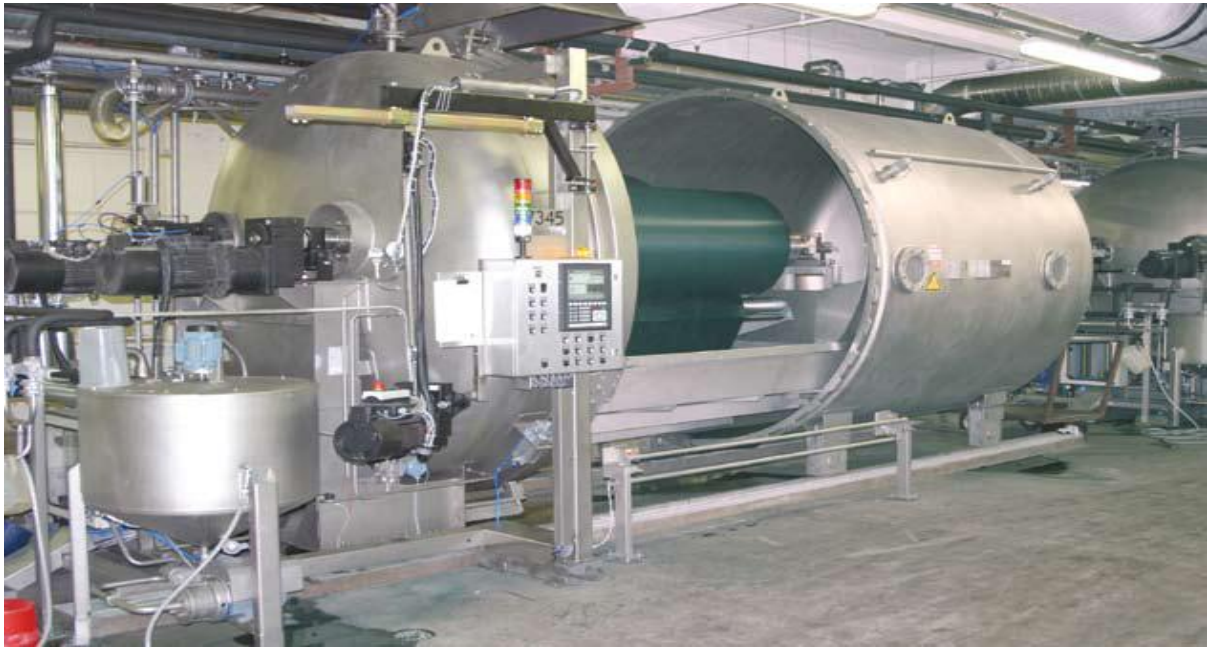
Modernized High Temperature Jigger machine
